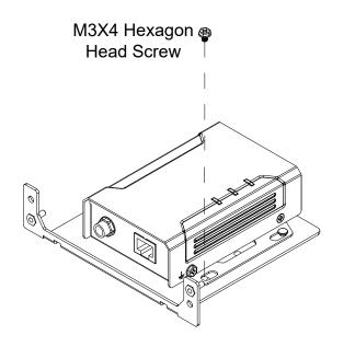
4. If the video extender doesn't have a mounting bracket, align the bottom holes and then screw the video extender to the mounting plate.
